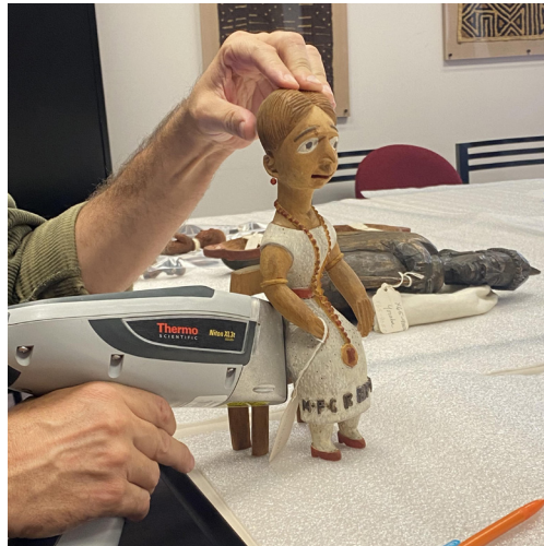
Christian de Brer uses a portable X-ray fluorescence spectrometer on a sculpture attributed to Odulate
