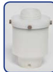
The 125 mL reaction vessel should be used for 0.5 - 5 mmol syntheses (up to 8 g of resin).
