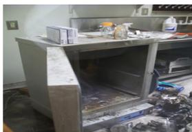
Lab ovens are used in research labs across the Emory Campus and although they are most commonly used for drying glassware, they pose significant health and fire hazards. Recently, an oven caught fire and caused fire and consequential water damage in the Claudia Nance Rollins School of Public Health Building. This simple fire has attributed to **\$60,000** worth of damage to the building. To avoid fires, explosions or other incidents adhere to the following when using laboratory ovens:
