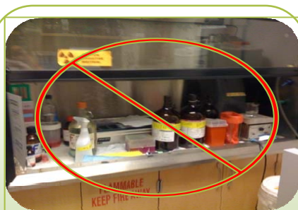
Excessive Chemical Storage Overcrowded and Cluttered
