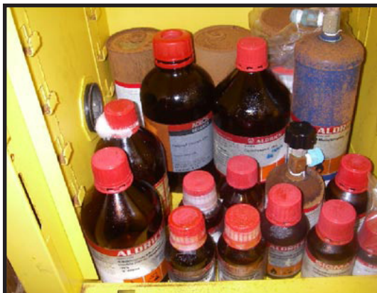
Image 1. Damage to the chemical containers and the cabinet due to incompatibilities.
