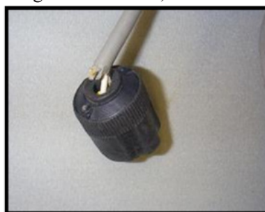
Image 1. Frayed Cord and Plug
